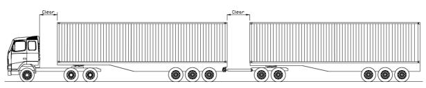
**4.2.3** The clear gap must be sufficient to enable the trailers to move through all the specified angles of rotation without contacting any other part of the towing vehicles, as per the following two diagrams. The red circles indicate the potential fouling zones.
