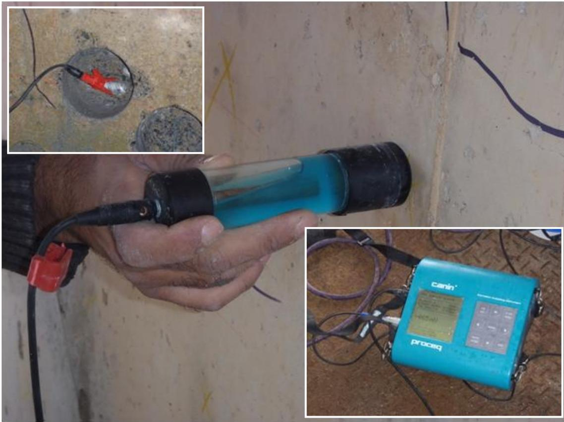
**Figure 13 - Typical Half-cell potential test showing electrode (centre), digital display box (bottom right) and connection with the reinforcement (top left)**
