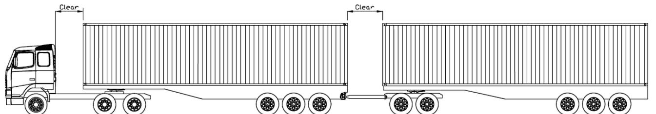
**5.5.3** The clear gap must be sufficient to enable the trailers to move through all the specified angles of rotation without contacting any other part of the towing vehicles, as per the following two diagrams. The red circles indicate the potential fouling zones.
