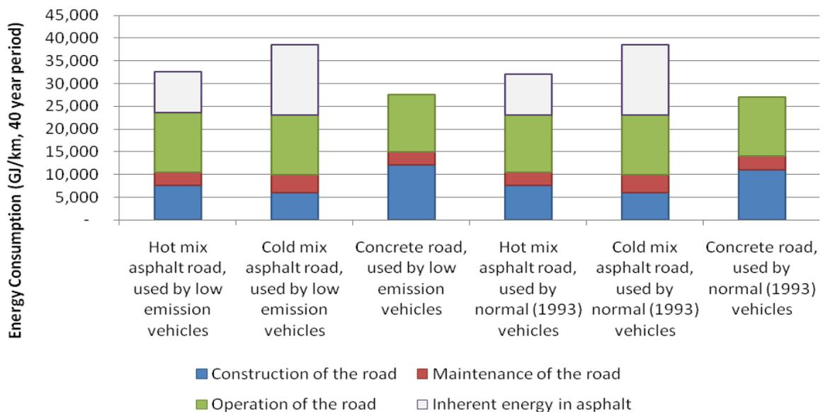
**Figure 3.5 Energy consumption for the road life cycle over a 40 year period**
