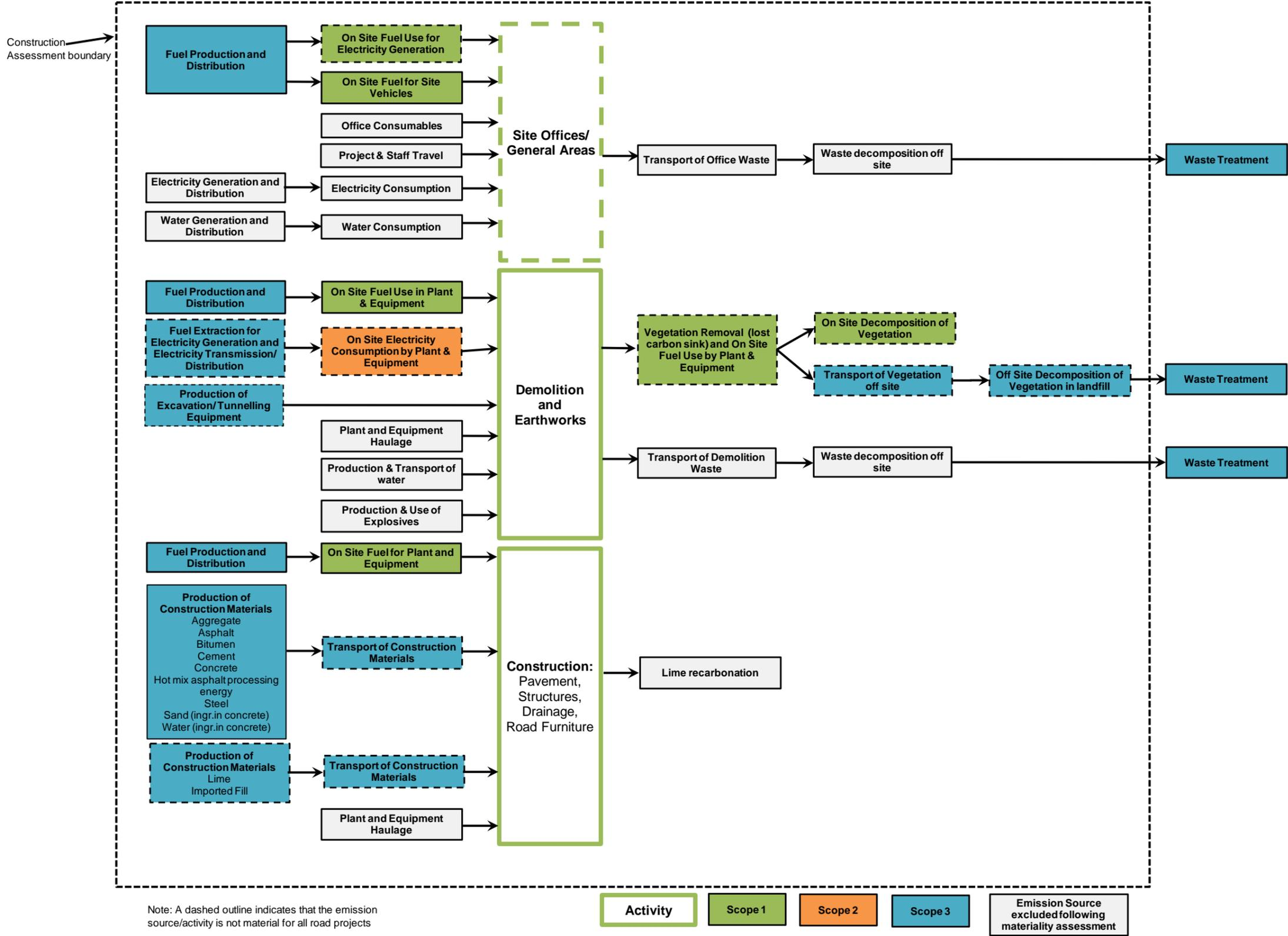
Figure 3.1 Complete Construction GHG Assessment Boundary
