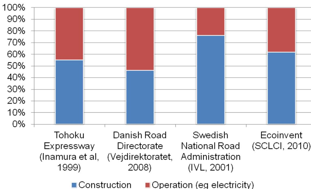
**Figure 3.4 Contribution of construction and operation to the GHG emissions for various road projects**
