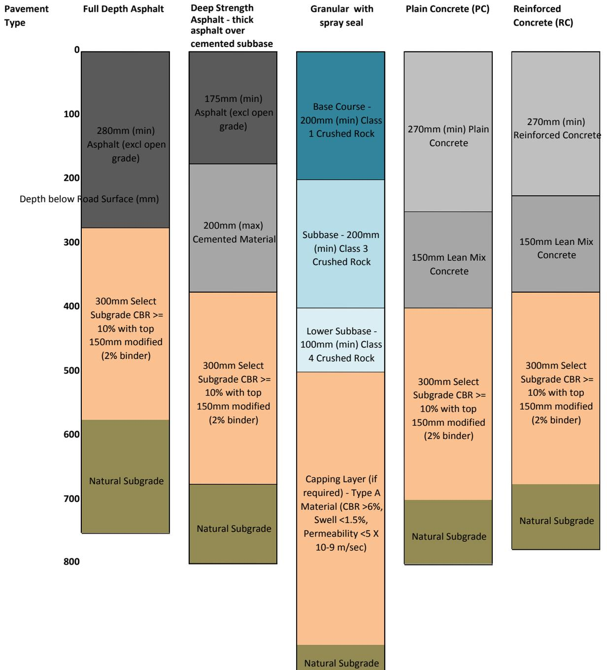
Figure 4.3 Pavement types and material depths
