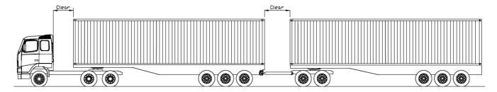
**5.5.3** The clear gap must be sufficient to enable the trailers to move through all the specified angles of rotation without contacting any other part of the towing vehicles, as per the following two diagrams. The red circles indicate the potential fouling zones.
