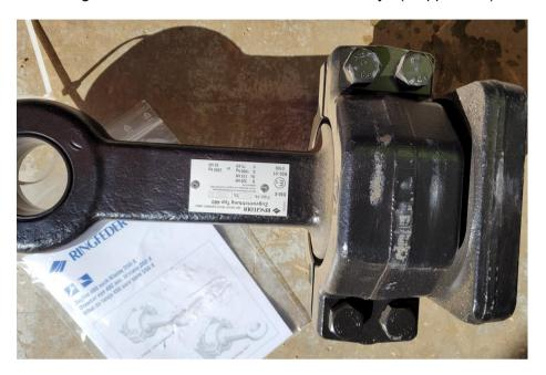
**4.2.10** Record the D-Rating, make and model for the Ringfeder (pin coupling) attached at the rear of the semi-trailer (if applicable).
