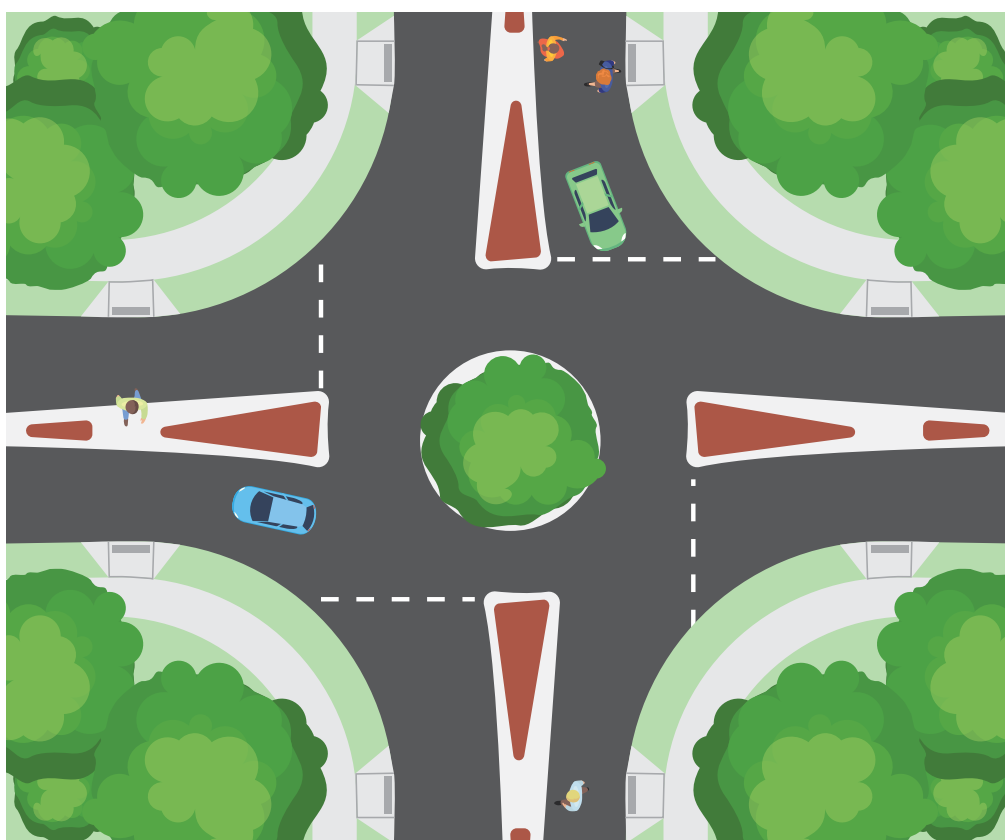
Figure 6-3 Unmarked crossings at single lane roundabout
