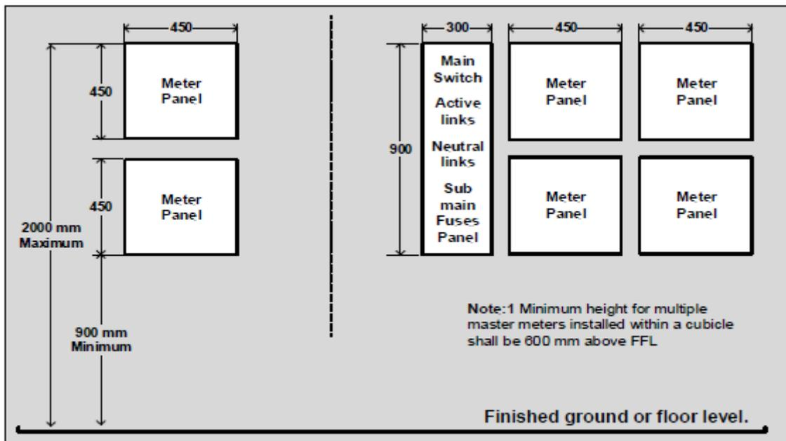
**Figure 22:** Typical multiple meter panel mounting heights
