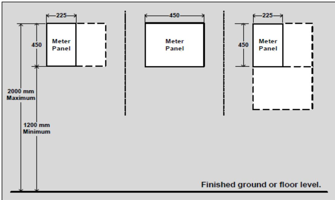
**Figure 21:** Typical meter panel mounting heights
