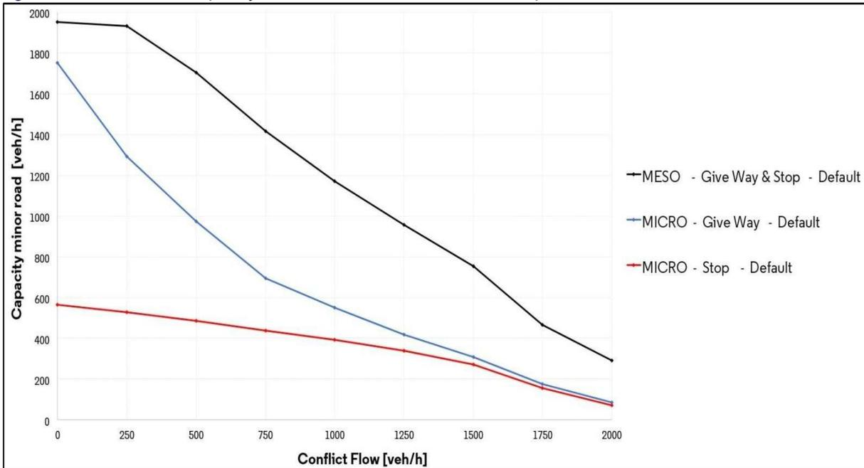
Figure 5-6: Two-way yield gap acceptance sensitivity in Visum (source: PTV, 2020)
