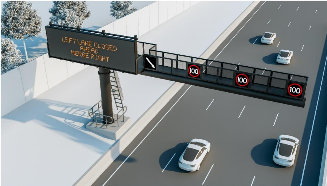
Figure 2-4: Tactical VMS on a Smart Freeway
