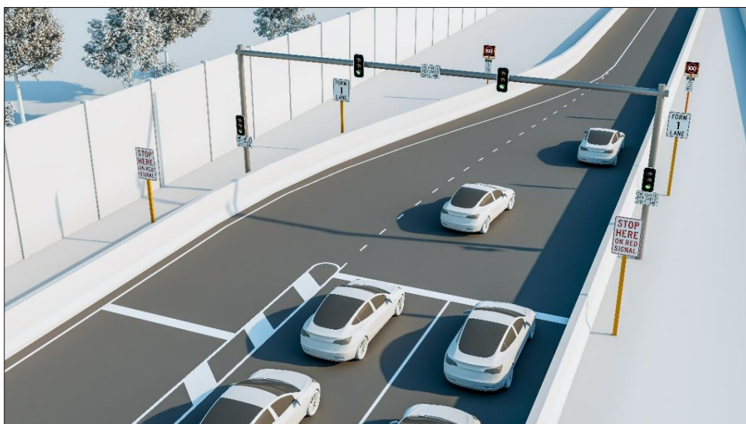
Figure 2-1: Coordinated ramp signals on the entry ramps of the freeway
