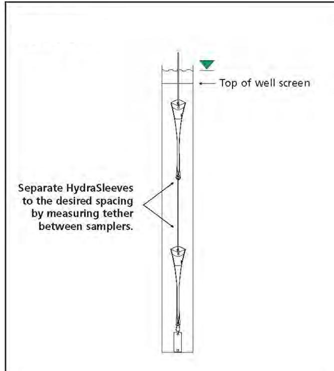
Figure 5. Alternative method for deploying multiple HydraSleeves.
