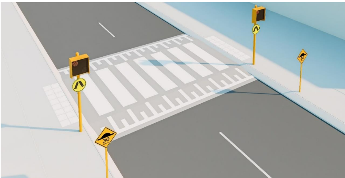
Figure 7-3: Example of position Wig Wags installed at an existing wombat crossing
