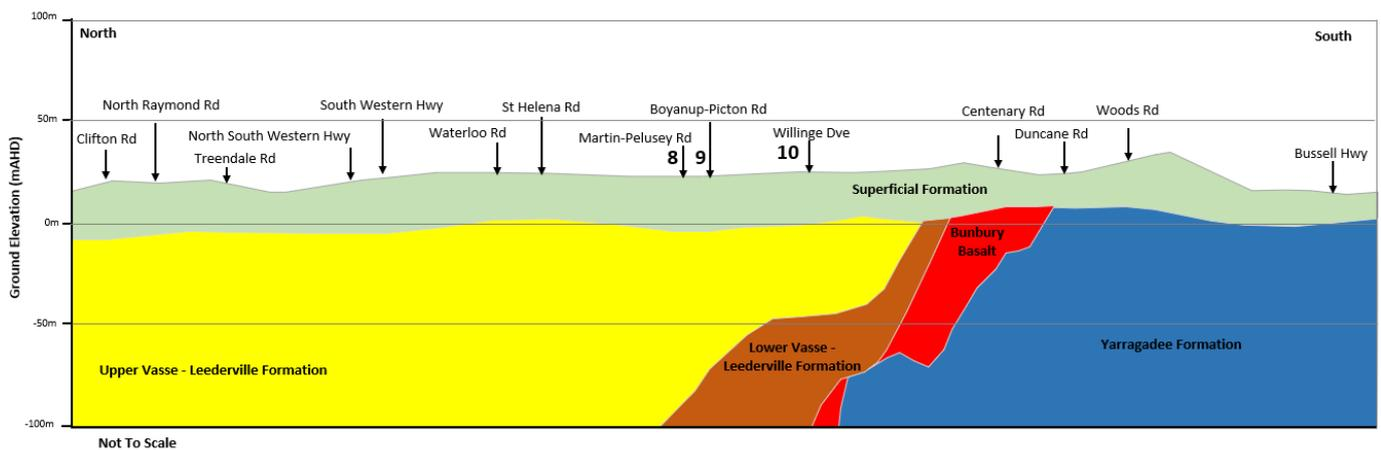
Figure 3. Hydro-stratigraphic schematic along the BORR alignment
