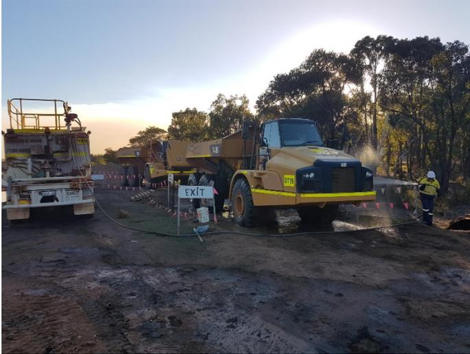
Photograph 2: Photograph of dieback cleaning station being used to clean machinery
