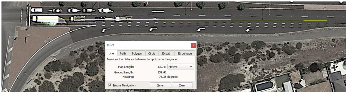
Figure 3-16: Free flow short lane length measurement example
