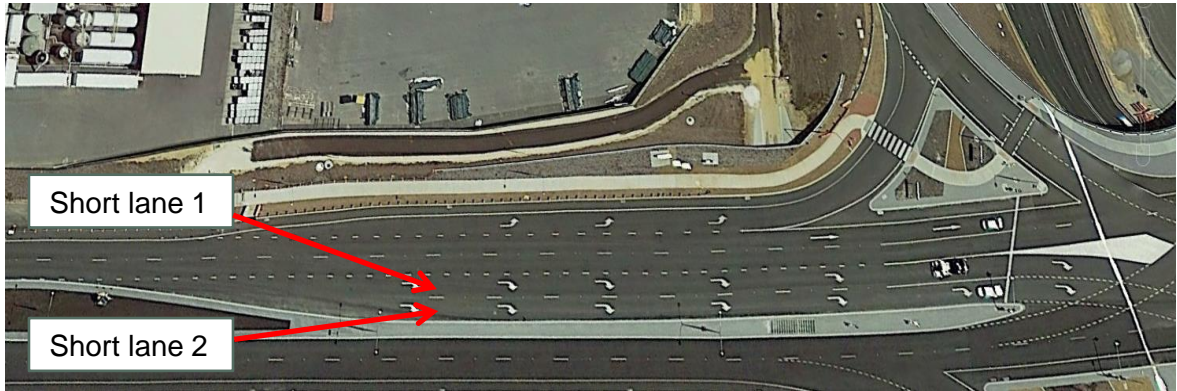
Figure 3-19: Typical double short lane layout
