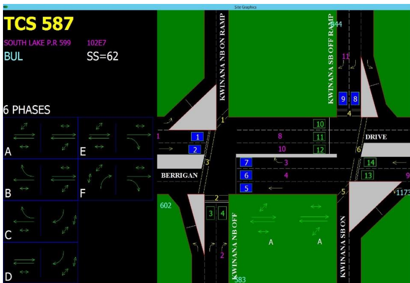
Figure 3-6: SCATS arms and loop numbers example for an interchange
