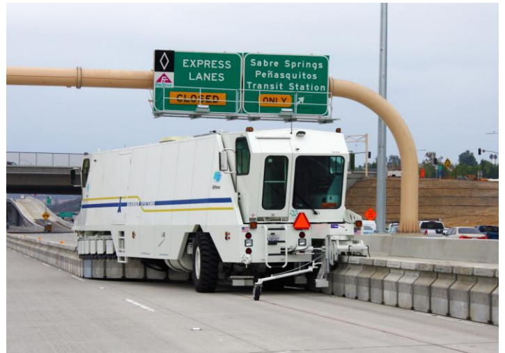
Photographs of typical Barrier Transfer Machines shifting barriers. Typical Permanent applications (left) and Typical Temporary or Construction applications
