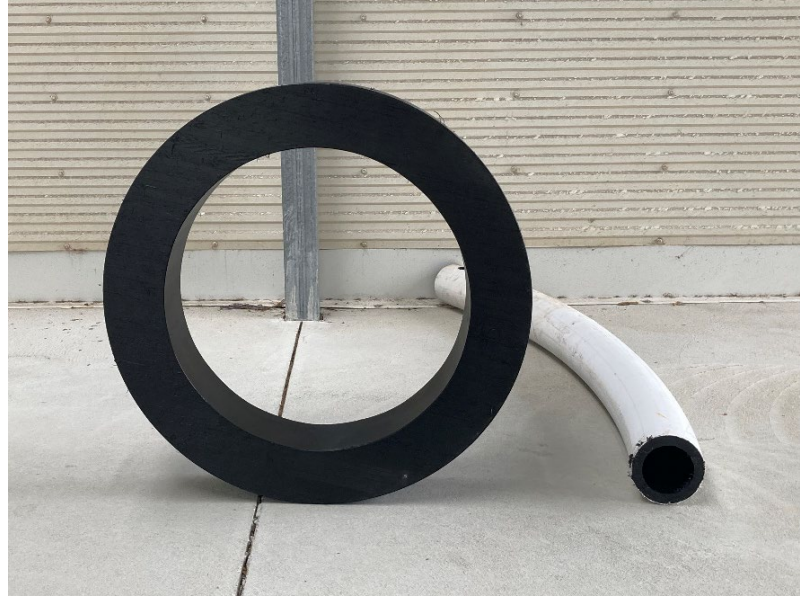
Picture 2: 630mm water pipe section (left) and 110mm telecommunications pipe section (right)
