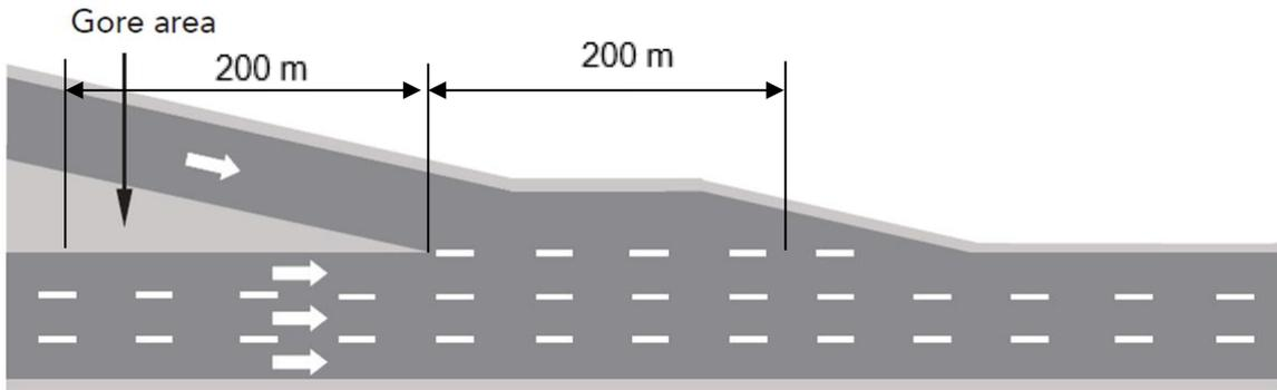
**Figure 7: Entry Ramp – desirable traffic volume within 200 m up and downstream of the start of the continuity line or lane line**
