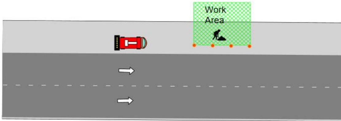
**Figure 13: Shadow vehicle scenario 2 – Works within 2 m of traffic lane.**
