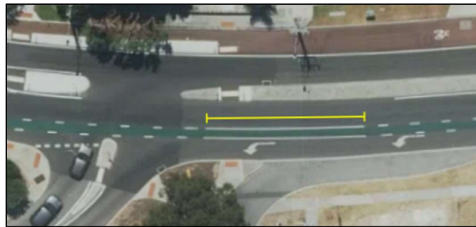
Figure 6.3 - Application of green surface treatment to the area between the left turn slip lane and side road (Hampton Road, Fremantle)
