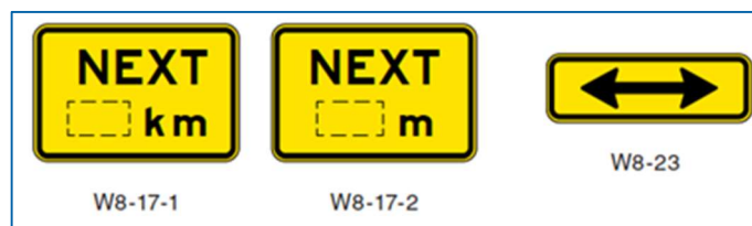
Figure 6.23 - Bicycle warning sign supplementary plates
