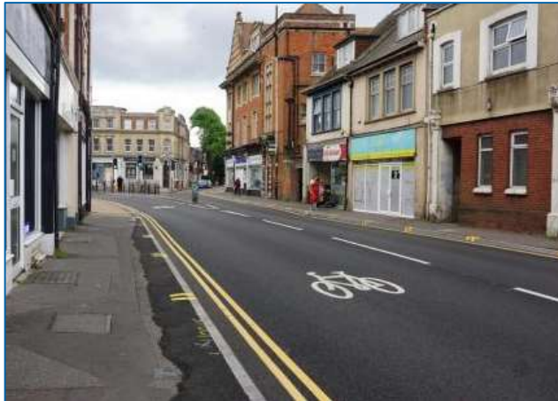
Figure 6.18 Bicycle pavement symbols applied in a residential local road environment (Boscombe, UK)
