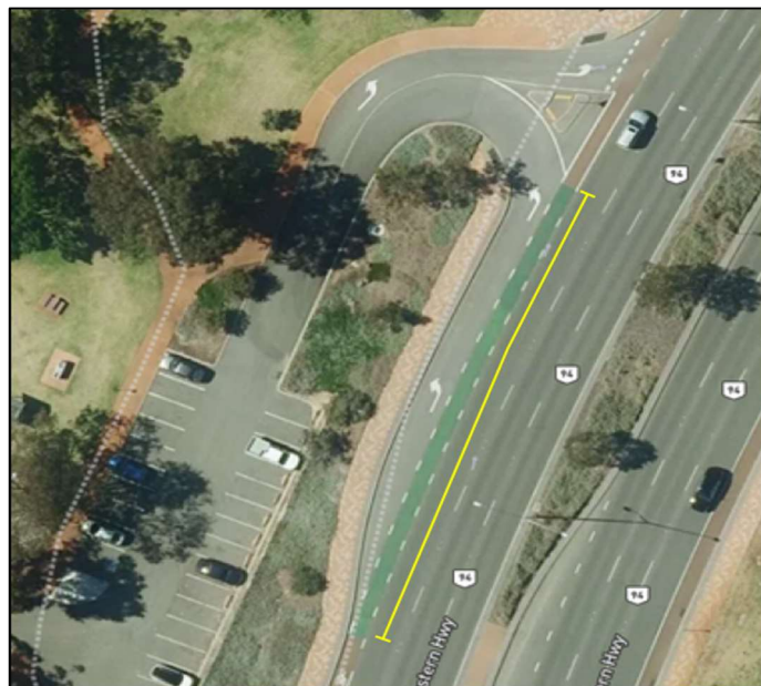
Figure 6.1 - Application of green surface treatment to left turn auxiliary lane (Great Eastern Highway, Belmont)
