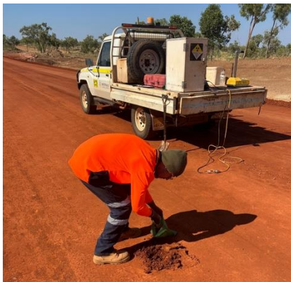
Sampling of road's subgrade for testing
