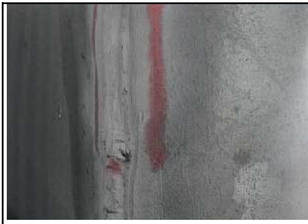
Photo No. 12: Sign connection 1 – close up of slag inclusions
