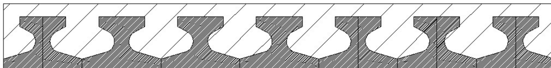
FIGURE E.2.2B - PRESTRESSED CONCRETE PRECAST INVERTED T-BEAMS WITH IN SITU INFILL
