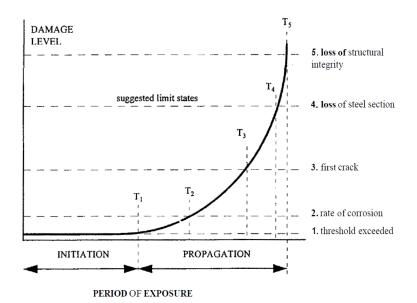
Figure G4 - Condition Limit states for deterioration caused by reinforcement corrosion (Bamforth and Pocock, 2000)
