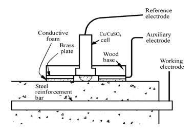
Figure 15 - Typical Three Electrode LPR Measurement
