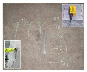
Figure 9 - TYPICAL COVER SURVEY
