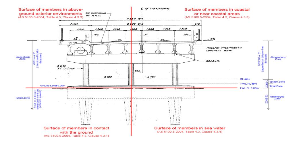
Figure F1 - Example Bridge Structural Components Exposure Classifications
