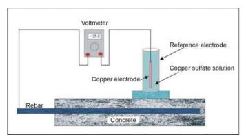
Figure 12 - Typical Connection of Half Cell Measurements
