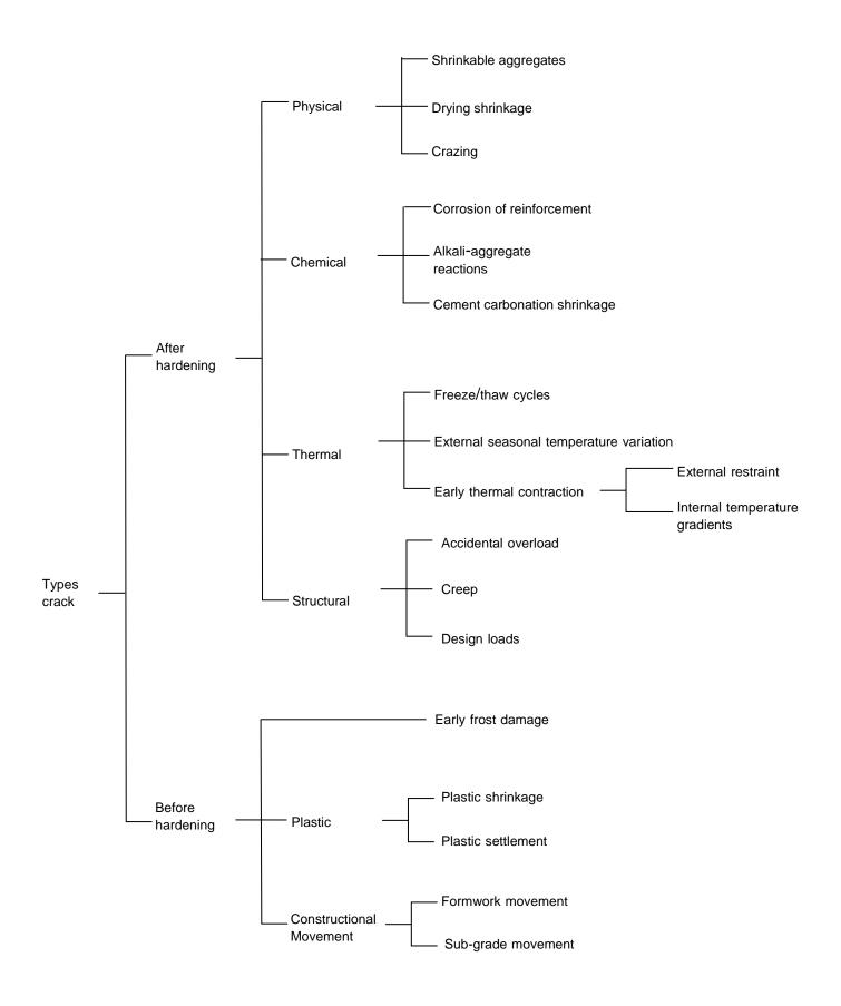
Figure 5 - Classification of cracks (Source HB 84-2006)
