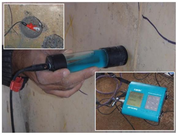
Figure 13 - Typical Half-cell potential test showing electrode (centre), digital display box (bottom right) and connection with the reinforcement (top left)
