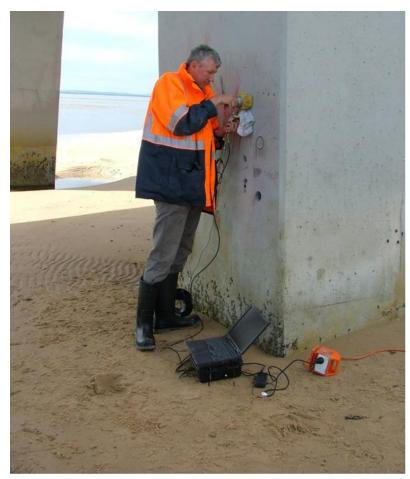
Figure 16 - Example of LPR Corrosion Rate test on Pier Leg
