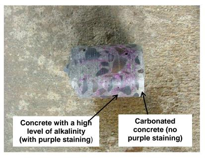
Figure 11 - TYPICAL CARBONATION TEST
