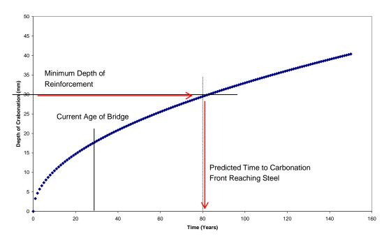
Figure G3 - Prediction of Depth of Carbonation vs Time
