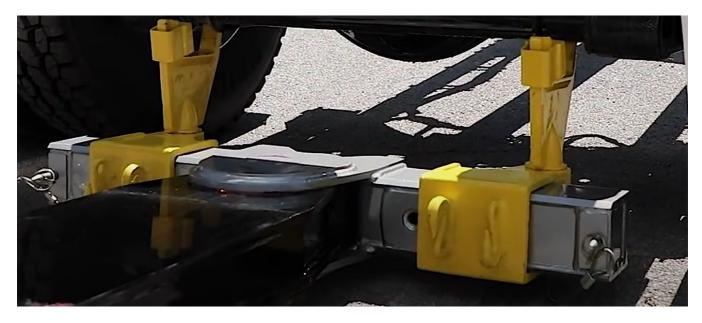
**5.3.2** The trailer must be secured to each underlift fork with adequately rated chains or straps.
