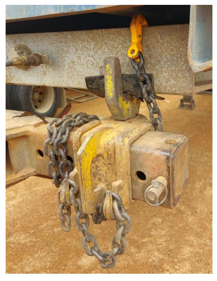
7.1.2 The semi-trailer must be secured to each underlift fork with adequately rated chains or straps.
