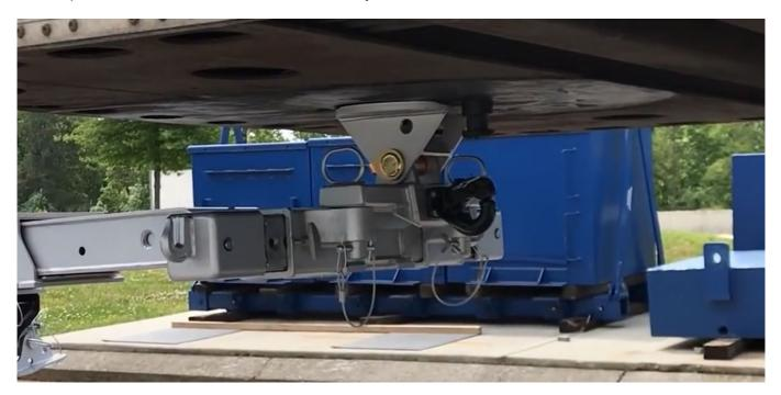
**6.1.2** The locking pin or locking pate must be fitted firmly across the king pin to prevent separation.
