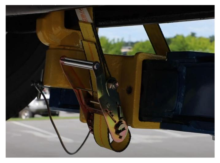
**5.3.3** Any rear axle(s) of the dog trailer that are still in contact with the ground must be chained up so there is sufficient ground clearance between the tyres and the road surface for towing.
