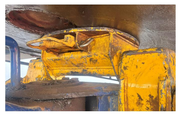
**6.1.3** Where the trailer does not have a block for a ballrace turntable, The underlift crossbar must be chained equally on both sides, or pinned, in a parallel position to prevent it from pivoting and allowing the trailer to articulate on the fifth wheel plate.
