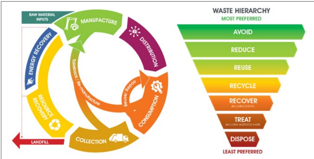
Figure 2: Talis Circular Economy Model, adapted from the National Waste Policy 2018 (left) and Waste Hierarchy (right)
