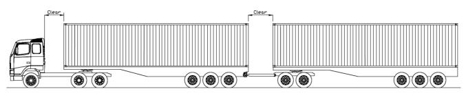
**5.4.3** The clear gap must be sufficient to enable the trailers to move through all the specified angles of rotation without contacting any other part of the towing vehicles, as per the following two diagrams. The red circles indicate the potential fouling zones.
