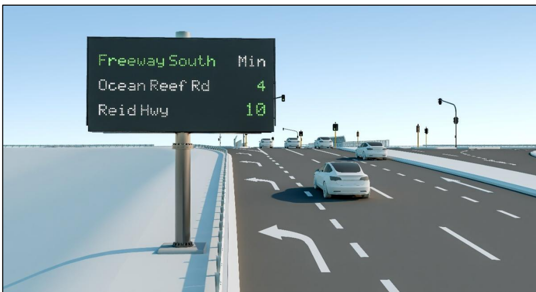
Figure 2-3: Real-time travel-time information displayed on arterial road RC3 on the approach to a Smart Freeway
