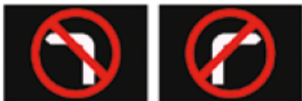
Figure 6-2: 'No Left Turn' and 'No Right Turn' symbols displayed on RC1 signs at arterial road / entry ramp intersections
