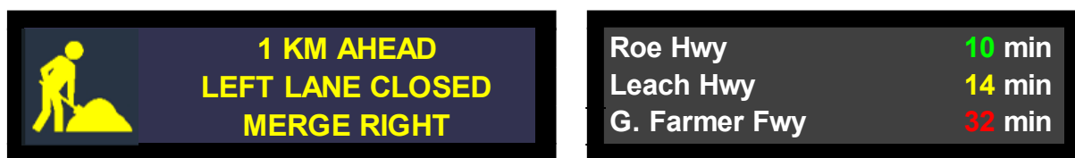
Figure 7-1: Strategic VMS incident message (left) and travel-times on Kwinana Freeway mainline (right)
