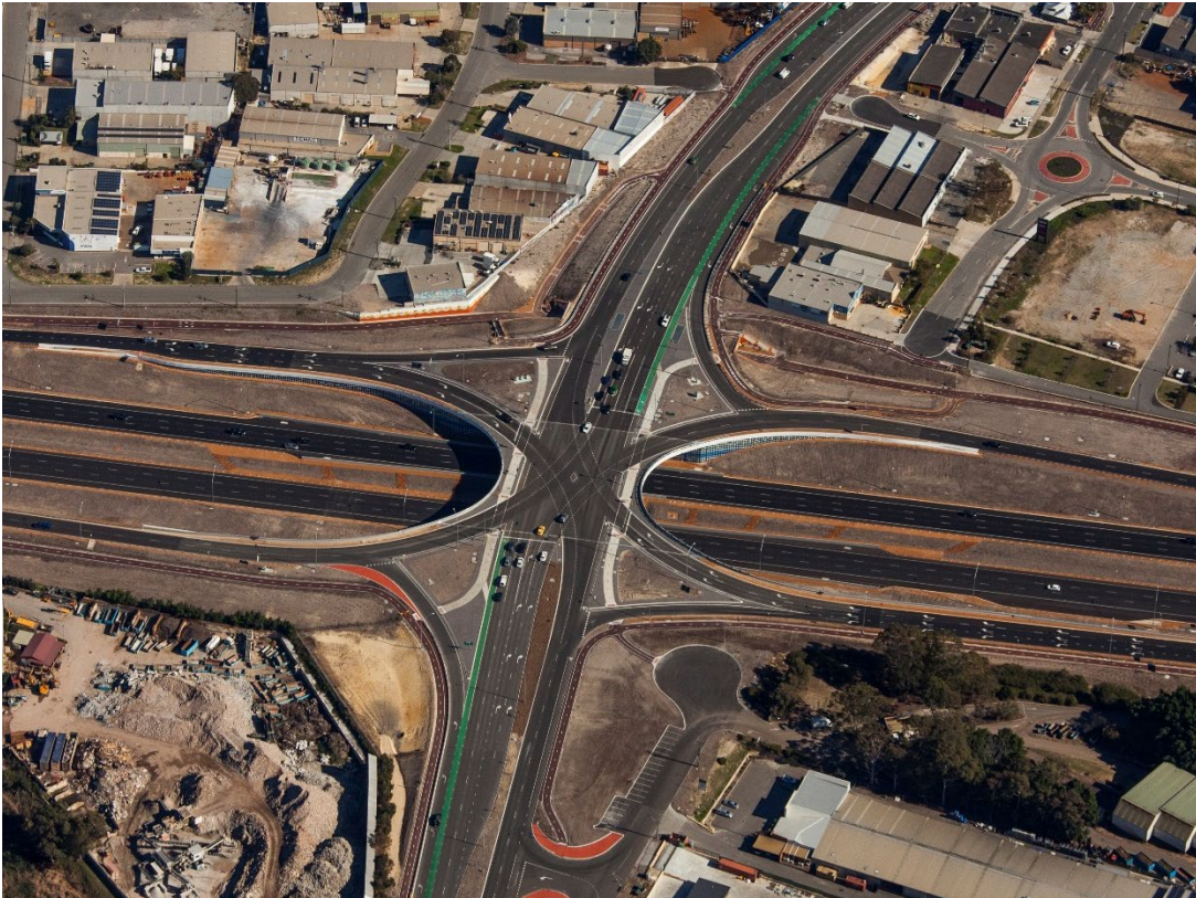
Figure 10-1 Example of single point urban interchange (SPUI)
