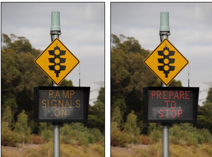
Figure 7-2 Example of alternating messages operating on an RC2 sign
