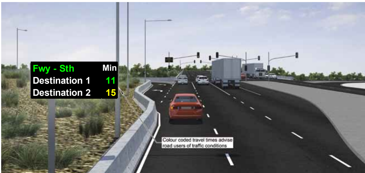
Figure 2-3 Real-time travel-time information displayed on arterial road VMS on the approach to the freeway
