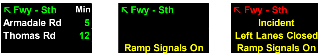
Figure 7-4 Examples of freeway-to-freeway VMS (RC3-C) displays (Roe Highway westbound traffic approaching Kwinana Freeway)
