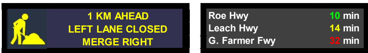
Figure 7-1 Freeway mainline VMS: incident message (left) and travel-times on Kwinana Freeway mainline (right)
