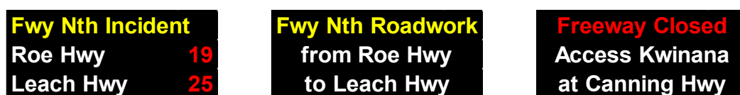
Figure 5-2 Examples of arterial road VMS incident and roadwork messages
