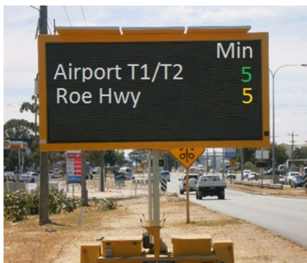
Figure 8-1 An example of portable VMS displaying travel time on a construction project
