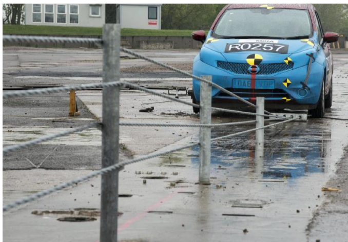
Photograph of MASH BRIFEN terminal end (installed in continuous concrete footing)
