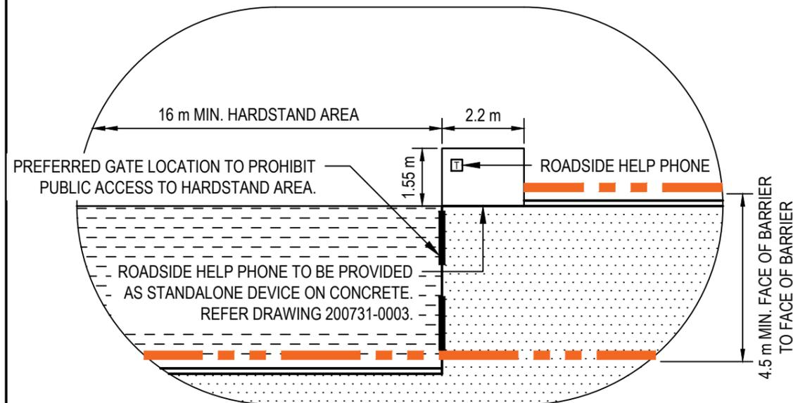
**TELEPHONE AND ACCESSIBILITY SLAB DETAIL
