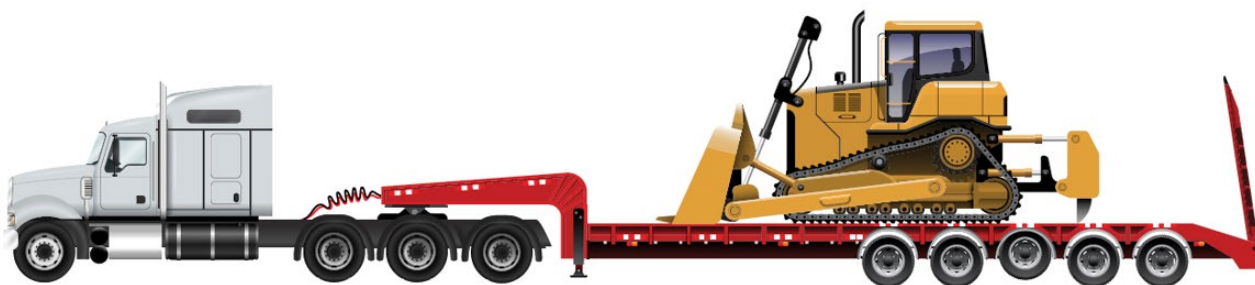
4 Axle Low Loader Trailer (lifting the 3 rd axle of a 5 axle Low Loader Trailer)
