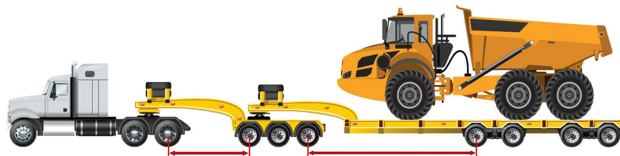
Axle Group Spacings: Rearmost Drive to Forwardmost Dolly, Rearmost Dolly to Forwardmost Trailer Axle
