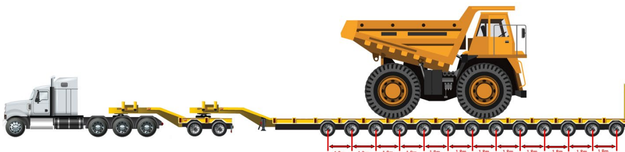
Platform Trailer Number of Axles: 13 Axle Spacings: 1.8
