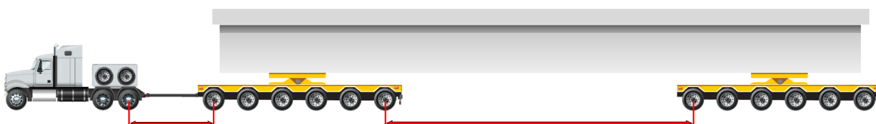
Split Platform Axle Group Spacings: Rearmost Drive to Forwardmost Trailer Axle, Axle Spacing to Rear Section
