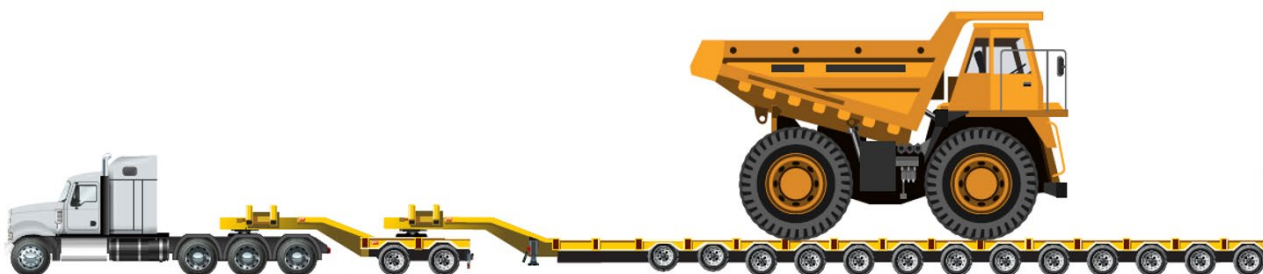
11 Axle Platform Trailer (lifting the 1 st and 2 nd axles of a 13 axle platform trailer)
