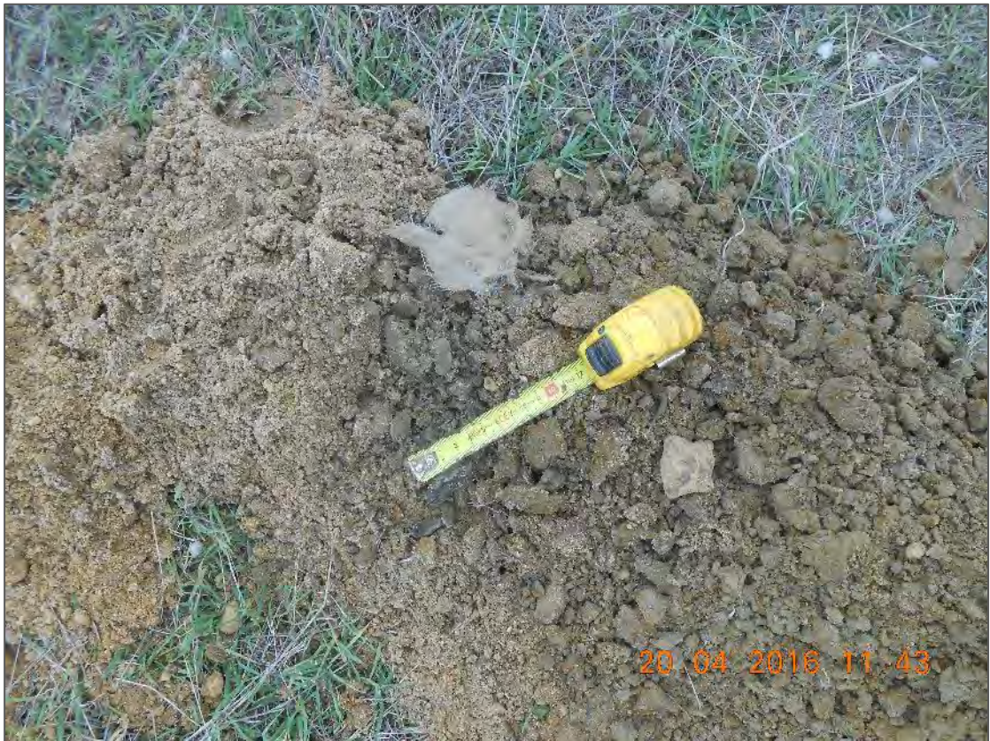
Photo 4: CH34600 geofabric evidence
