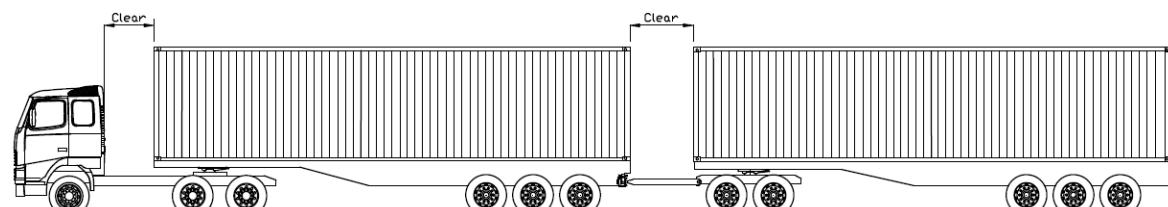
**11.3.3** The clear gap must be sufficient to enable the trailers to move through all the specified angles of rotation without contacting any other part of the towing vehicles, as per the following two diagrams. The red circles indicate the potential fouling zones.
