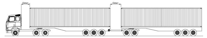
**4.5.3** The clear gap must be sufficient to enable the trailers to move through all the specified angles of rotation without contacting any other part of the towing vehicles, as per the following two diagrams. The red circles indicate the potential fouling zones.
