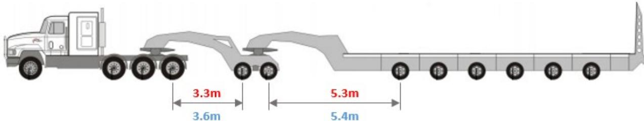
**Prime mover to dolly** axle spacing is compliant as the variance between the specified axle spacing of 3.3m and the measured axle spacing of 3.6m is 300mm (not more than 300mm).
