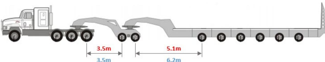
**Prime mover to dolly** axle spacing is compliant as it is equal to the axle spacing specified on the permit.
