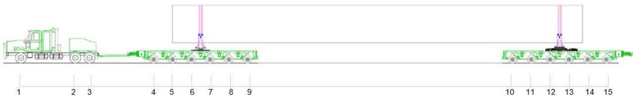
Axle spacing measurements are to be taken from the centre of the axle to the centre of the adjacent axle. Alternatively, axle spacing measurements can be taken from the outside of the rim to the same position on the outside of the rim on the adjacent axle, provided the rims are the same diameter.
