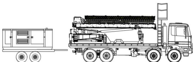
**Note:** 12.0 tonne permitted on the Twin Steer Axle Group where it is fitted with load sharing suspension and tyres  $\geq 375$  mm. Statutory mass limits apply to all other axle groups.
