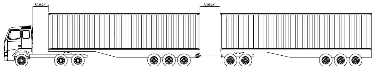
**6.4.3** The clear gap must be sufficient to enable the trailers to move through all the specified angles of rotation without contacting any other part of the towing vehicles, as per the following two diagrams. The red circles indicate the potential fouling zones.
