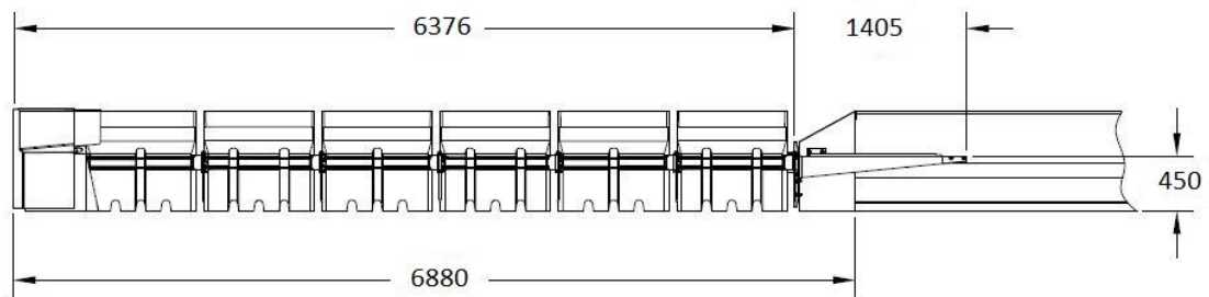
Elevation: Absorb 350 TL 2 (70km/h), Six Element System
