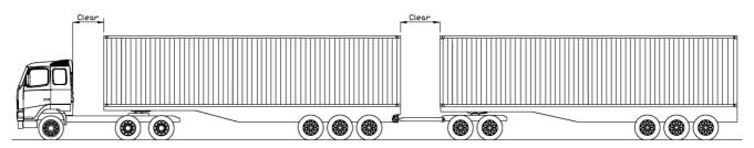
**5.4.3** The clear gap must be sufficient to enable the trailers to move through all the specified angles of rotation without contacting any other part of the towing vehicles, as per the following two diagrams. The red circles indicate the potential fouling zones.
