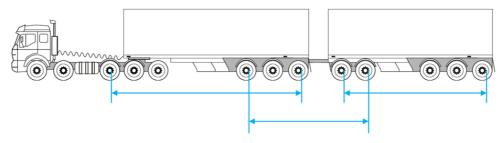
"Single Axle" does not include a single steer axle.
