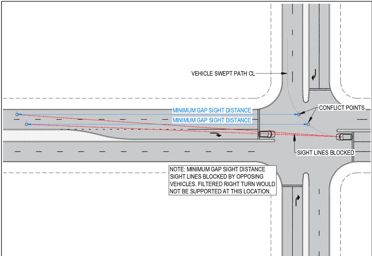
**Figure 3.8: Minimum Gap Sight Distance (MGSD) - Failing**
