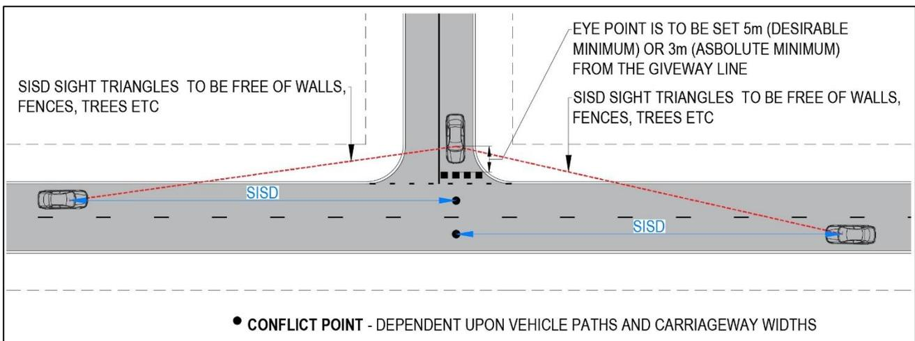
**Figure 3.2 (Plan Only): Safe Intersection Sight Distance (SISD)**
