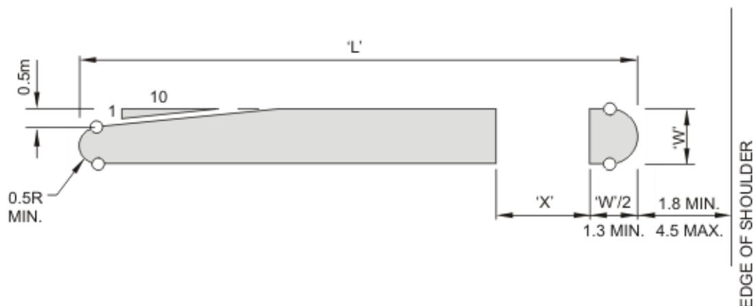
**Figure 6.1: Splitter Island Geometry**
