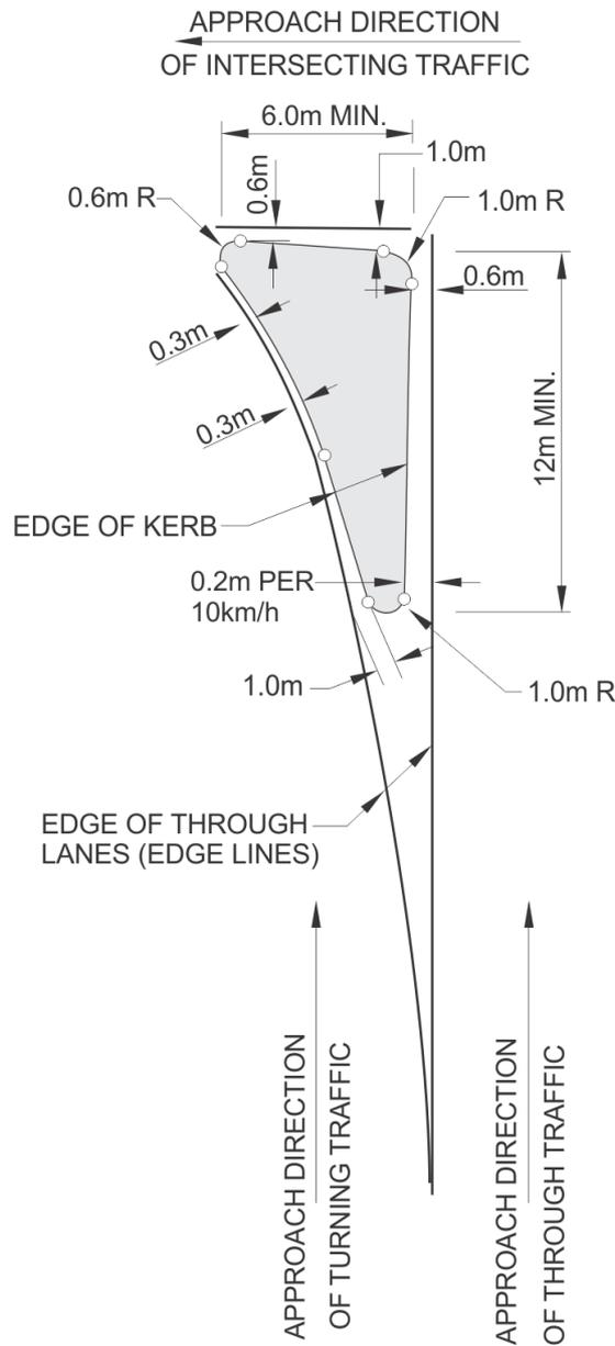
**Figure 6.18: Left Turn Island for Signalised Intersections**
