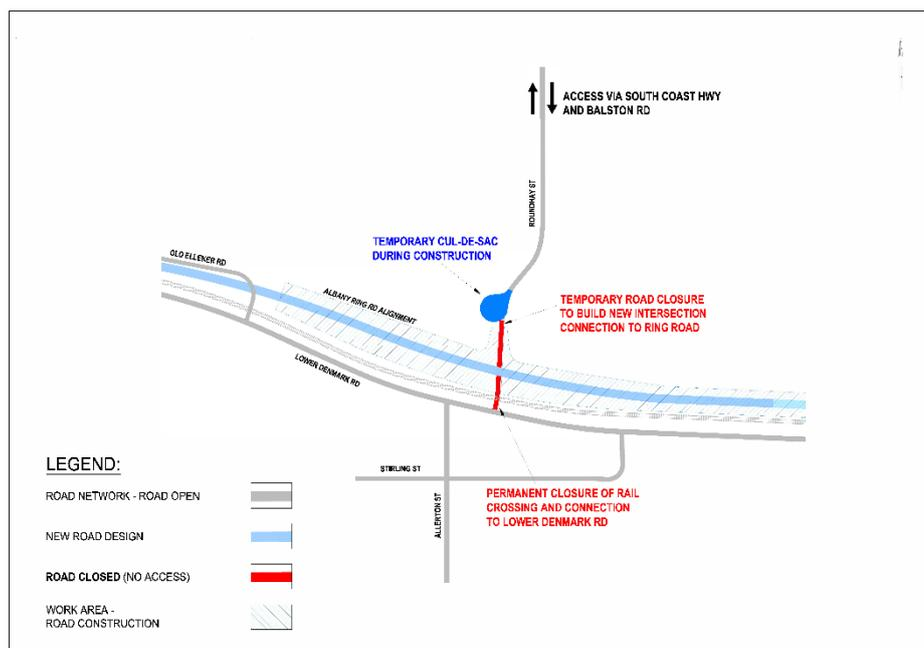
Figure 1: Access changes during construction
