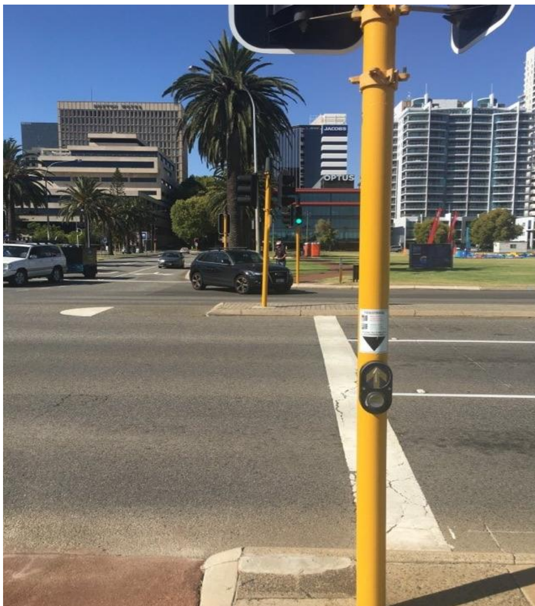
Figure 8: An example pedestrian crossing with no pedestrian aspects, with a traffic roundel display for pedestrians
