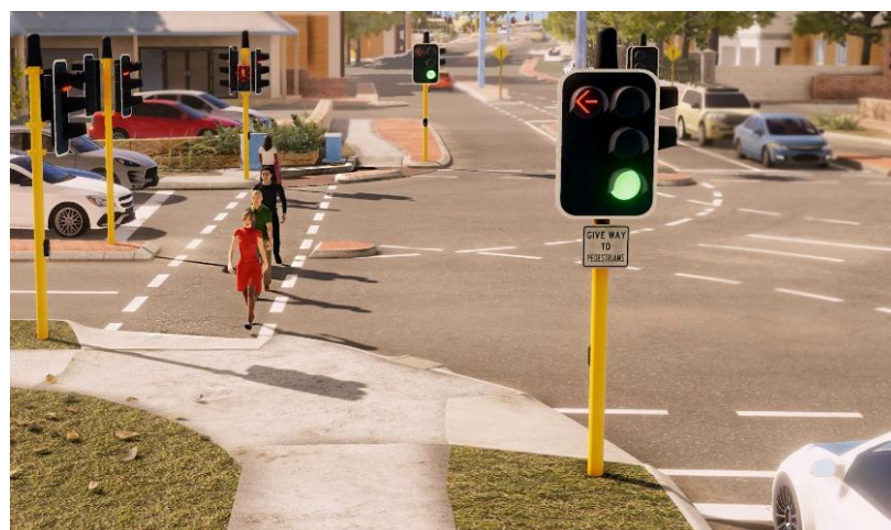
Image 8: Flashing red symbol Clearance Time and red arrow display for vehicles for duration of crossing movement
