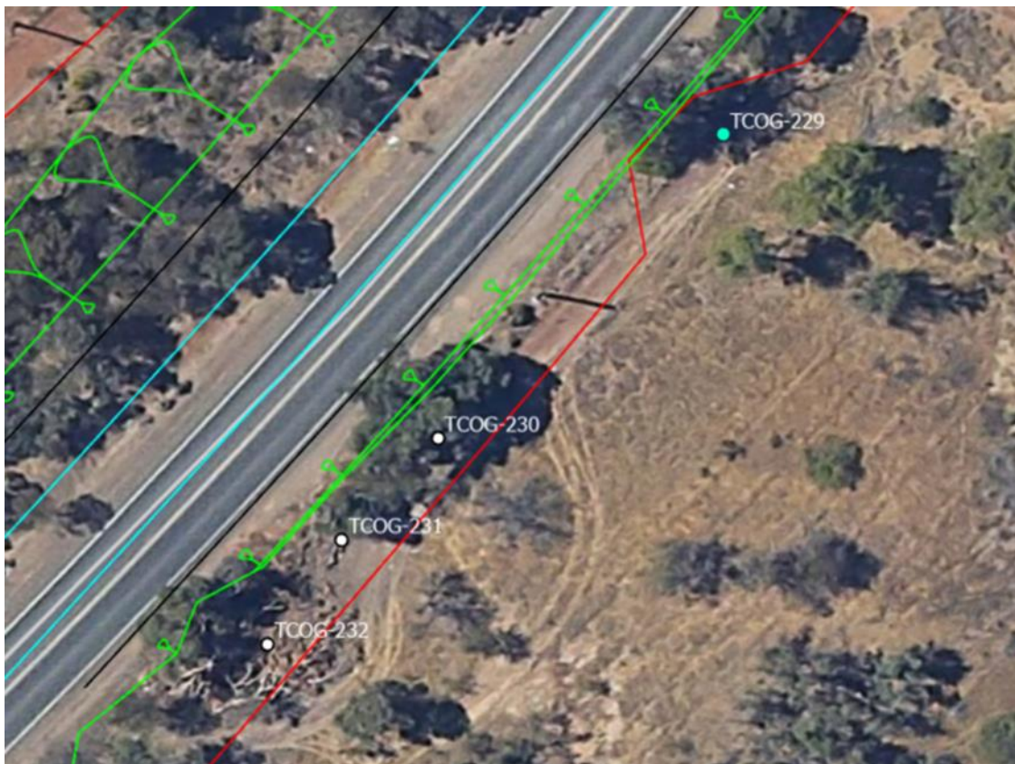
Figure 3-3(a) Installation of crash safety barriers (solid double green line on southern side of road) to avoid tree with a hollow of suitable size for Black Cockatoo breeding (TCOG – 229) and other suitable DBH trees.
