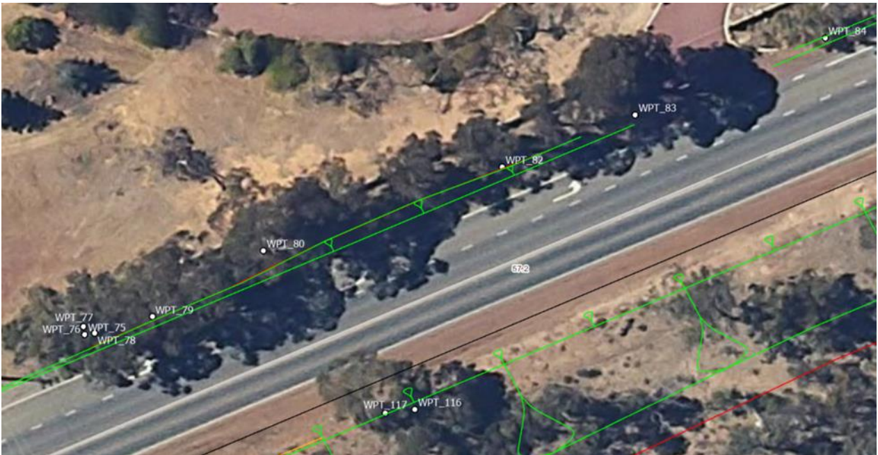
Figure 3-3(c) Shifting alignment to one side and utilising existing road drainage network to minimise impact on suitable DBH trees.
