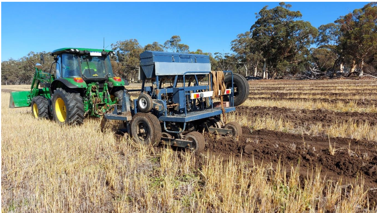
Plate 1 A CommVeg direct seeder in operation at example Main Roads revegetation site in the Wheatbelt region of Western Australia.
