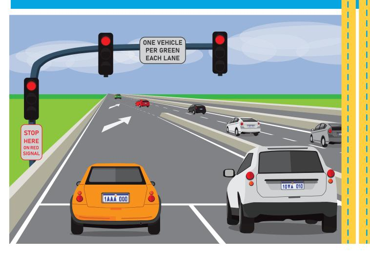
Perth's Smart Freeway has modified traffic lights as ramp signals on five northbound on-ramps, between Farrington Road and Cranford Avenue. New technology will co-ordinate these ramp signals to help vehicles merge more easily and keep the freeway flowing.
