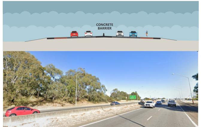
In locations where there are constraints on both sides, such as development or environmental issues, a narrow median with concrete barrier would minimise impacts.
