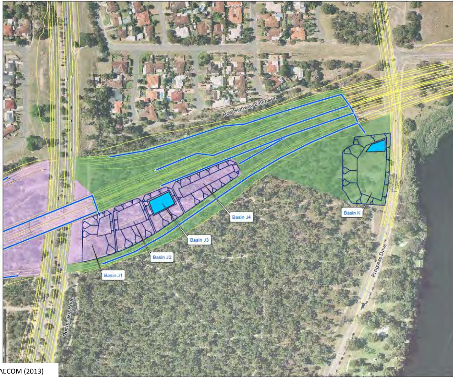
Figure A7: North Lake Rd/ Roe Hwy Interchange Basin Plan
