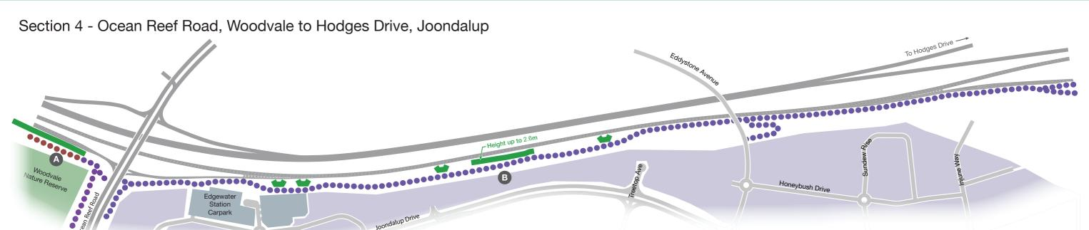
Retaining wall heights are from the lowest ground level. Noise wall, and combined noise and retaining wall heights are from the Principal Shared Path.
